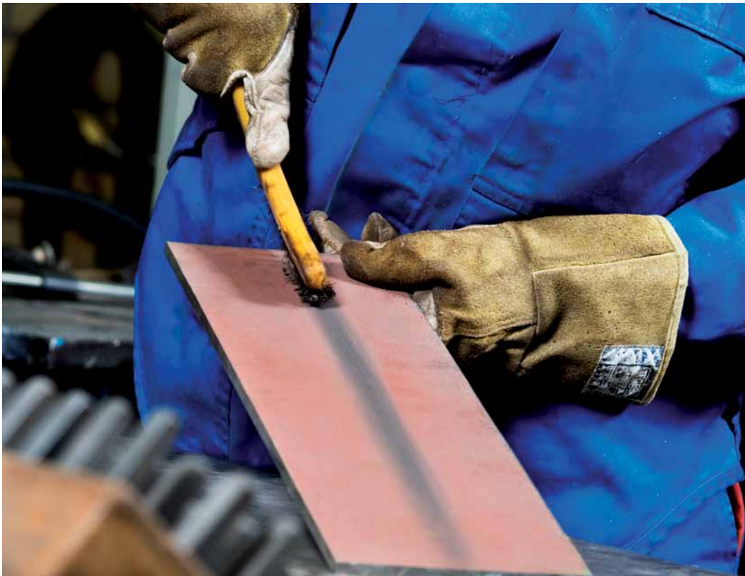
Figure 13: The primer is easy to brush away if necessary
